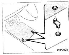
Use a floor mat of the correct size. If the vehicle carpet and floor mat have 2 holes, then they are designed for use with locking clips. Attach the floor mat to the vehicle carpet using the clips. Lock the clips into the holes in the vehicle carpet.
