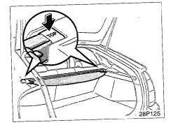
To replace the luggage cover, adjust the cover so that "TOP" is facing upwards.
