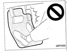
/ CAUTION Make sure the floor mat is properly placed on the vehicle carpet. If the floor mat slips and interferes with the movement of the pedals during driv ing, it may cause an accident.
